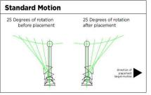
This is standard rotary placement motion without the influence of a cam. The product is placed on the target with no forward motion.
